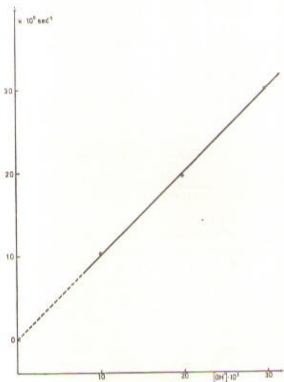
Figure 2. Plot of 10^6 k against 10^2 [\text{KOH}] , 65 \pm 0.02^\circ\text{C} . Solvent 32.0 mole percent DMSO.
