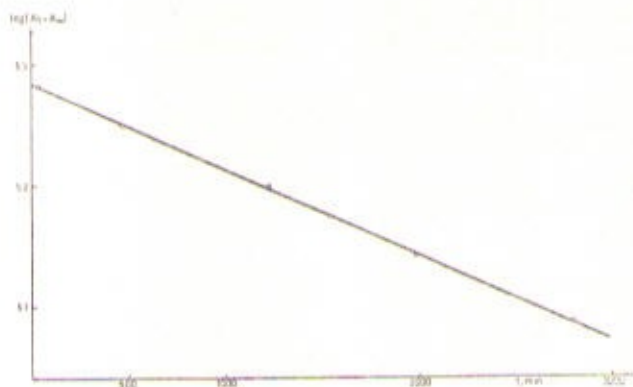
Figure 1. Determination of the exchange rate constant. Plot of \log(A_t - A_\infty) against time. A_t and A_\infty counts per aliquot per 10 minutes at times t and infinity, respectively. Solvent 32.0 mol percent DMSO, temperature 65 \pm 0.02^\circ\text{C} . Catalyst 0.3 M KOH. The exchange rate constant k is 2.73 \times 10^{-6} \text{ sec}^{-1} .
