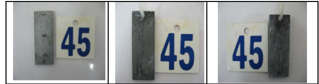
Figure 1. Samples without appearance of corrosion after 2160 hours in salt spray chamber
